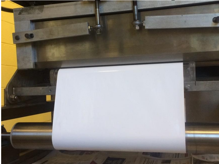
14" Amine Coating on ZY Layer on PES
